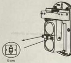
The accuracy of beam alignment turns higher when the red LEVEL indicator becomes brighter.
